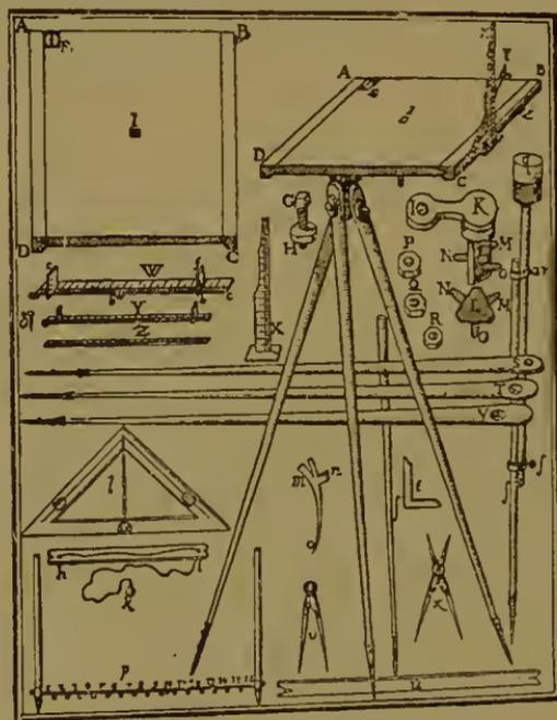
Fig. 14.—Pretonius's Plane-table.
